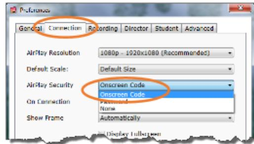
Also under the "Connections" tab, Change On Connection to Connect and Hide Device.
